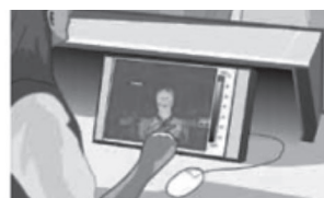
Step 2: IR camera operator looks at a color monitor that shows audible and/or visible color alarms when an individual shows an "out of norm" body temperature.
