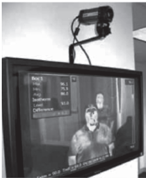
Fixed-mount FLIR A320 with the color alarming in progress
