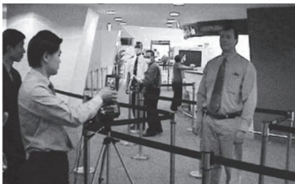
Setting up a FLIR IR camera with Automatic Temperature Compensator (ATC) for elevated body temperature detection
