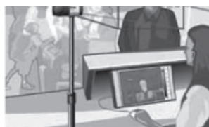
Step 1: Individuals are remotely monitored as they pass a screening checkpoint set up at an airport, border, or in the entrance lobby to a corporation or school.
